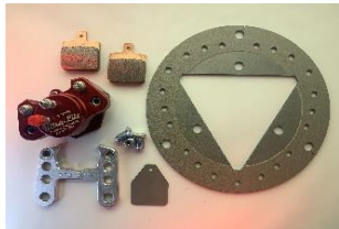
410-7100 1 -C-250-9875-3 Rotor-Steel-Solid .250" x 9.875" - 3 Bolt, 3- 980-6000 Rotor Bolts, 1- 140-1005/140-1006 100 Series Caliper - Floating Mount (1) - 1.625" or 1.5" piston, 1 - 930-0255 Caliper Bracket - Left Front Sprint with (2) .220" Spacers, 2 - UL-104 Pad - Left Front Sprint 589A Compound, 1-170-0104 Heat Shield - Titanium - .065" Thick
